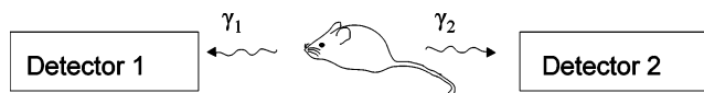
Figure 30. In vivo ^{111}\text{In} PAC experiments on mice. Meares and Westmoreland 101 have used time-integrated PAC on ^{111}\text{In} -labeled compounds in living mice. The mouse was placed in the barrel of a slightly modified 60 mL syringe. Thereby, the time development of ^{111}\text{In}^{3+} bound to EDTA, citrate, chloride, and nitrilotriacetate could be followed in living mice.
